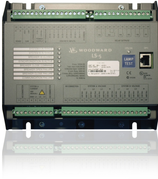
LS-511 - Sheet metal housing. Back panel mounting.
